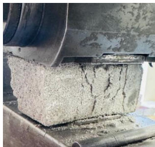
Figure 2: Foamed concrete specimen under the compressive strength testing machine.
