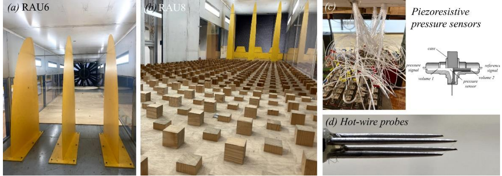
Figure 2: (a) Configuration RAU6 in ABL wind tunnel at Ruhr University Bochum; (b) Configuration RAU8 in ABL wind tunnel at Ruhr University Bochum; (c) Apparatus for pressure measurements; (d) Hot-wire probe for velocity measurements
