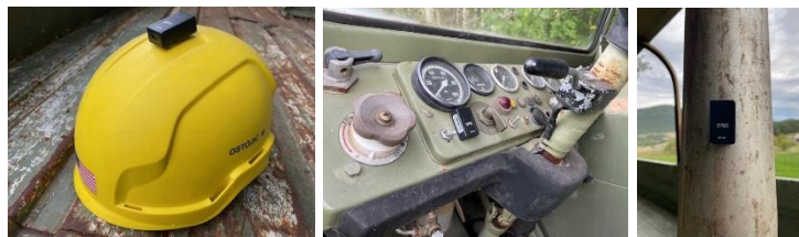
Figure 3: GPS-based tracking system applied to the worker (a), equipment (b), and structural element (c) (source: authors' research)
