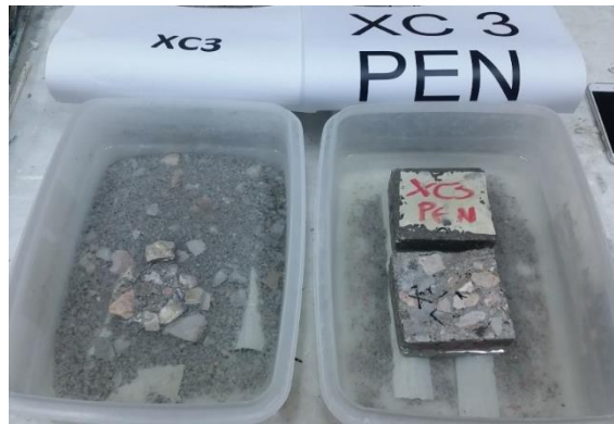
Figure 1: Final view of XC3 concrete specimens after completion of 15 cycles
