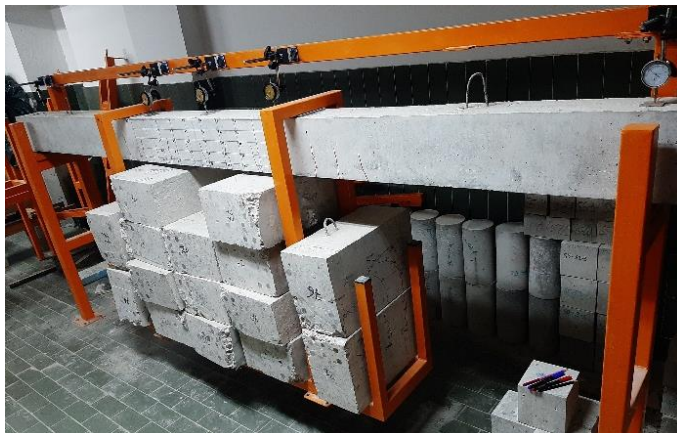
Figure 9: Experimental setup: four-point bending test
