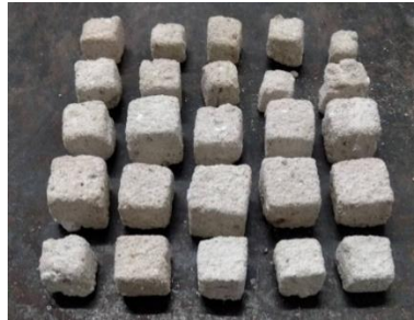
Figure 2: Processed specimens of mortara
