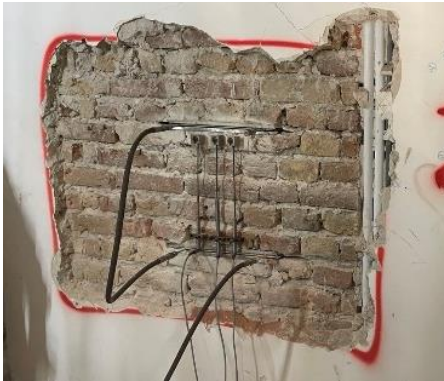
Figure 6: Test arrangement for determining the modulus of elasticity
