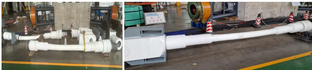
Figure 12: Post-test inspection of the hanger specimens and anchorage assemblies
