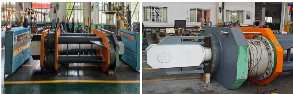
Figure 9: Full-scale static tensile test arrangement: fixed-end anchorage (left) and longitudinal view of the assembled hanger specimen (right)
