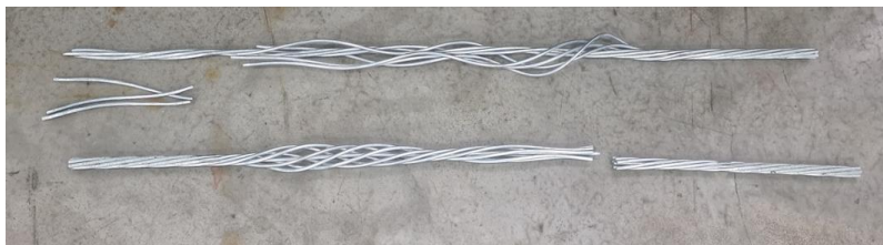
Figure 11: Individual strand specimen after tensile testing, showing characteristic wire fractures
