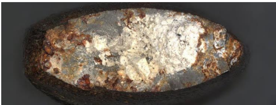
Figure 7: Wire break with mortar at the fracture surface (photo: BAM Berlin, [19])
