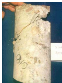
Figure 8: Crack within the concrete of RC columns affected by the fire
