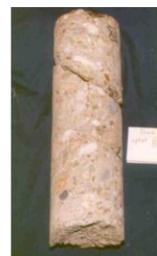
Figure 8: Crack within the concrete of RC columns affected by the fire
