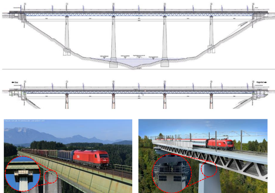
Figure 2: Existing Jauntal Bridge, strengthened reinforced concrete substructure and new composite steel–concrete superstructure
