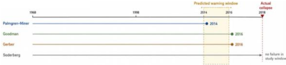
Figure 3: End-of-life estimates obtained from the Morandi corrosion-fatigue assessment
