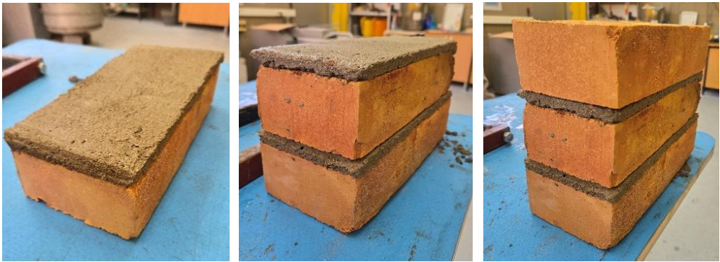
Figure 2: Sample preparation for testing shear strength
