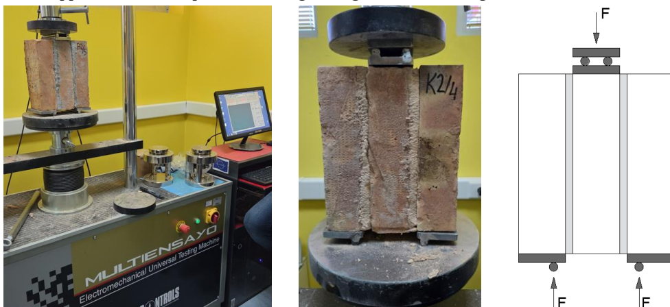
Figure 5: Shear strength testing of mortar joints
