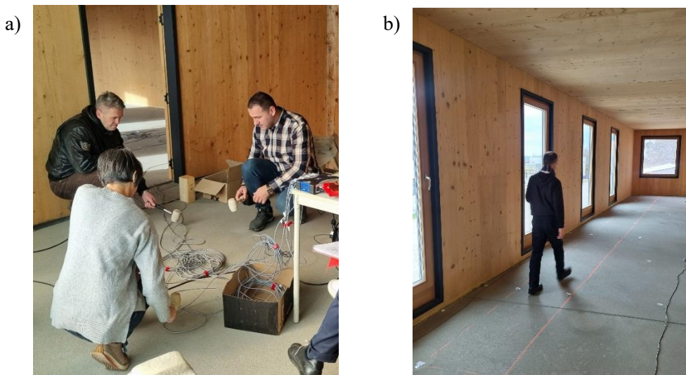
Figure 3: a) Experimental testing of modal properties and b) an example of a walking test
