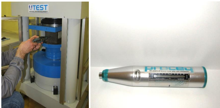
Figure 4: Schmidt hammer rebound number testing (left); Appearance of the Schmidt hammer
